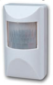
Our 1/4" color CCD camera is encased in a white PIR housing. It has a 1.0 lux sensitivity with 350 line resolution. It features a 3.6mm wide angle pinhole lens and built-in electronic shutter. A 12V DC power supply is included. A B/W version of this camera can be found under model number VL-265PIR and VL-272PIR (with working PIR). A fully adjustable wall/ceiling mount is included with this unit.
